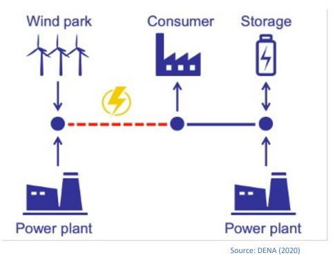
Used at overloaded grid points, batteries can prevent renewable energy generators from being shut down.
