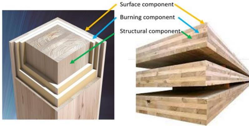
Figure 3-7: Examples of new wood materials in Japan
