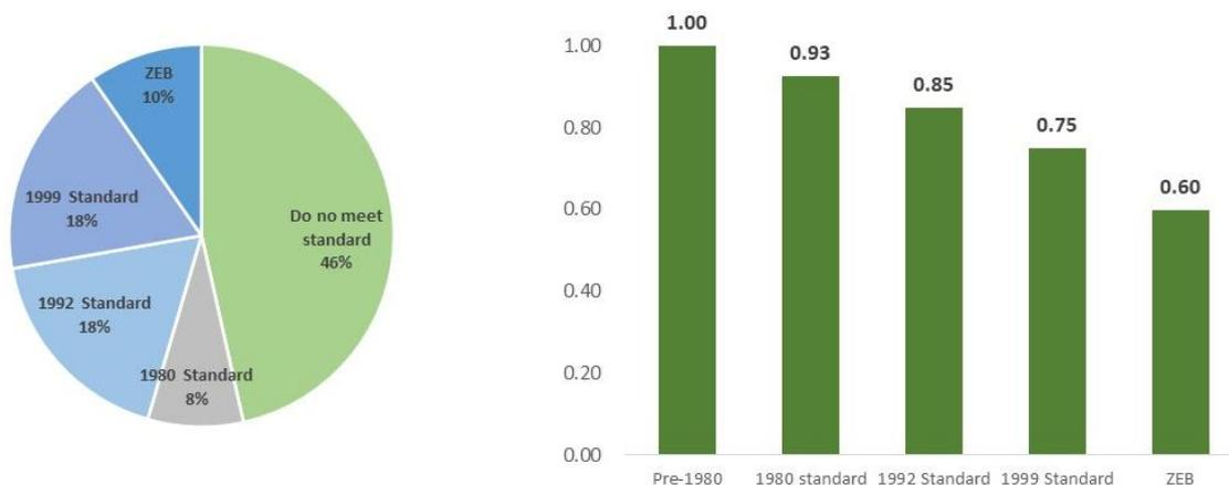
Figure 2-11: (Left) Thermal Insulation performance of non-residential building stock (FY2017) (Right) Relative Non-residential Building Insulation Performance
