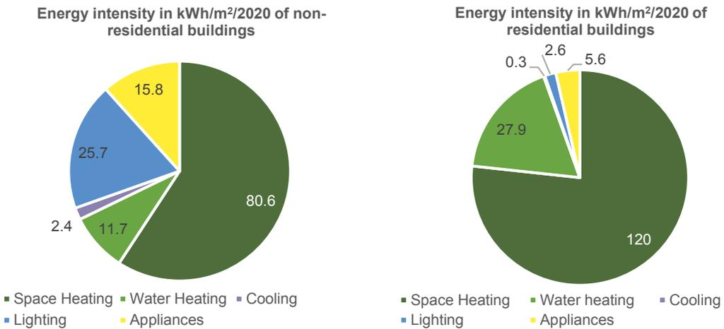
Figure 2-12: Final energy intensity of non-residential and residential buildings, overall and by end use
