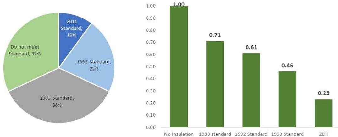
Figure 2-10: (Left) Thermal Insulation performance of about 50 million housing stock (FY2017) (Right) Relative Housing Insulation Performance
