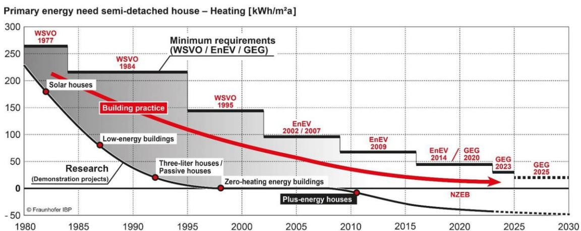
Figure 3-2: Evolution of energy performance requirement for a common type of new residential buildings
